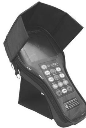
**Fig. 2.3 Usage of blend for avoiding glares on the protection glass.**
