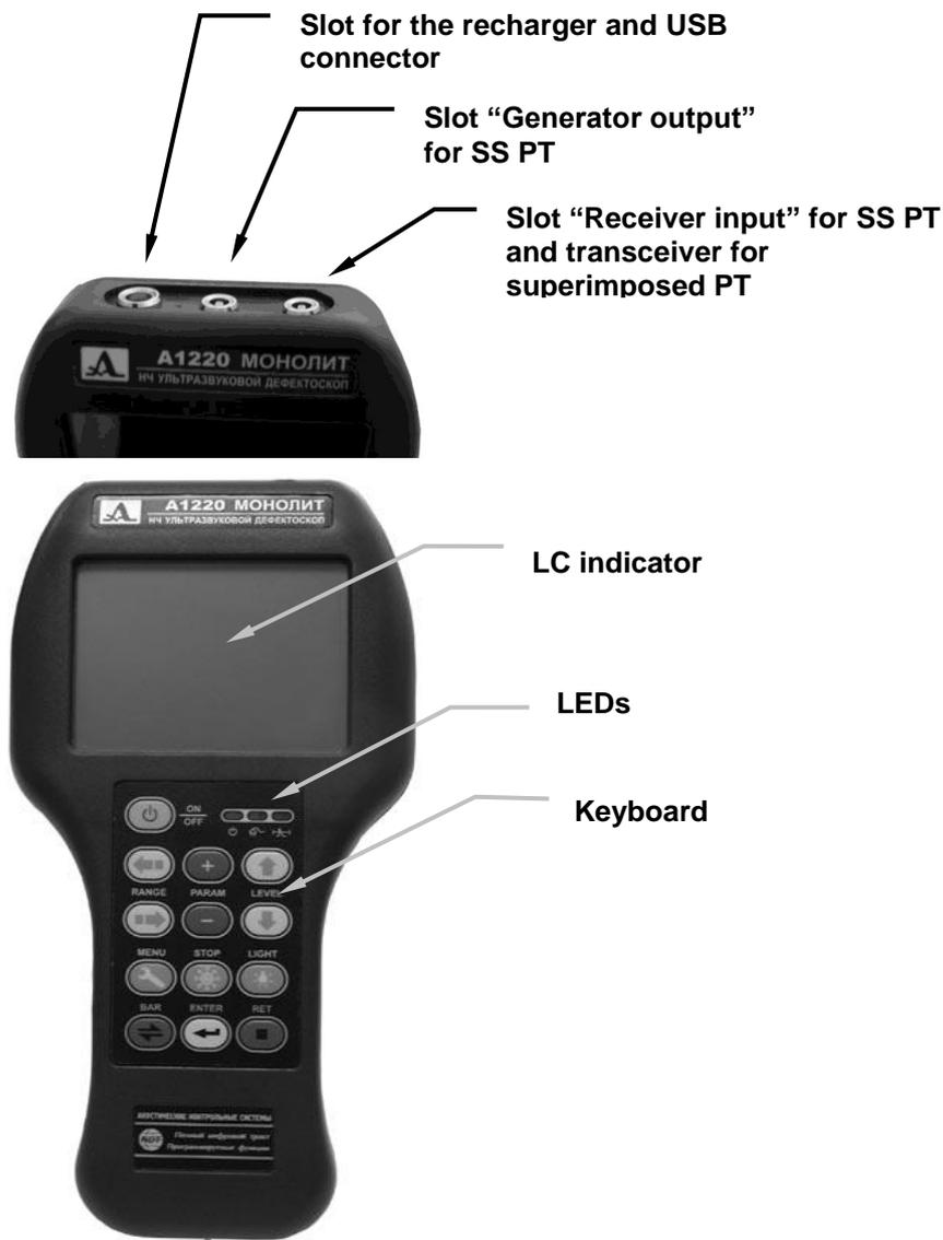
**Fig. 2.1. Flaw detector electronic block**
