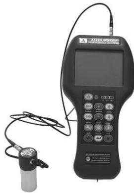
The unary cable shall be connected to the slot not marked by the red spot.
