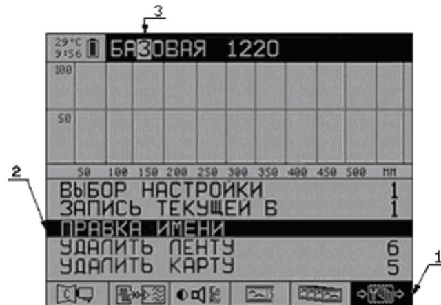
**Fig. 4.2 Screen in MENU mode. Configuration name change**
