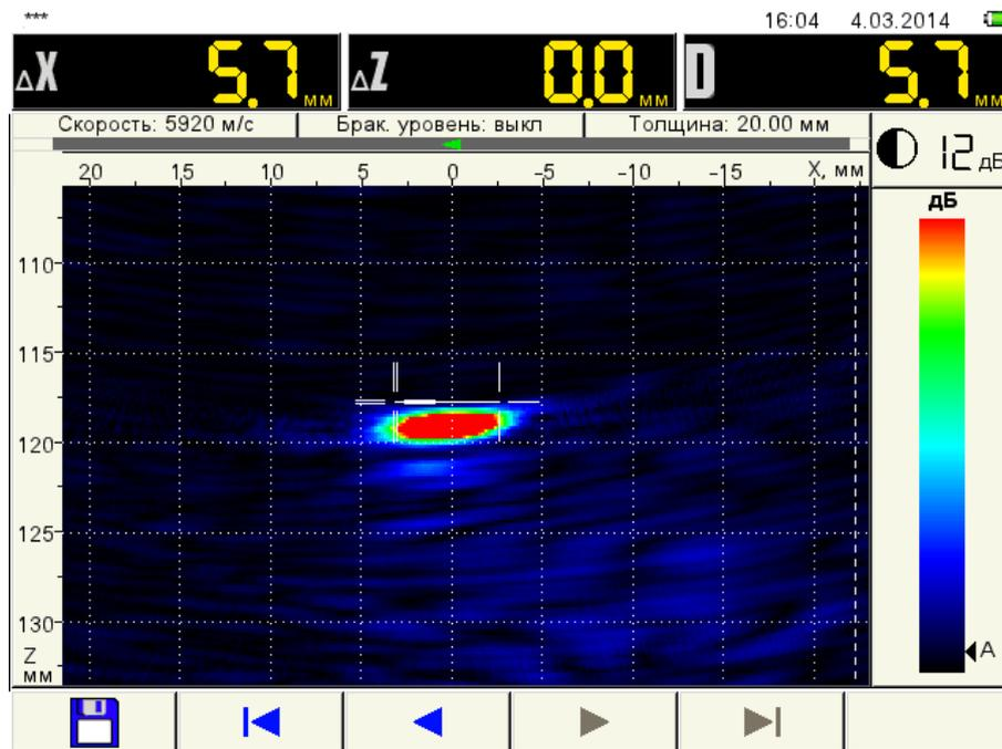
Figure 38 Measurement of the front length of defect
