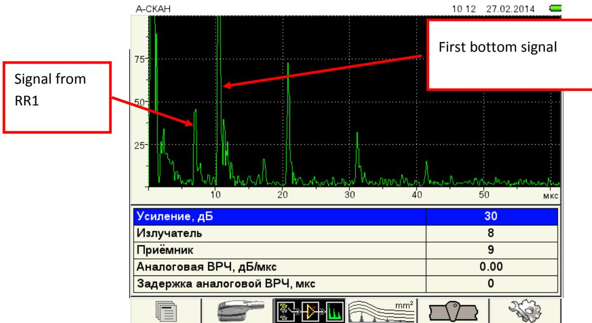
Figure 12 Third tab of the Configurations mode
