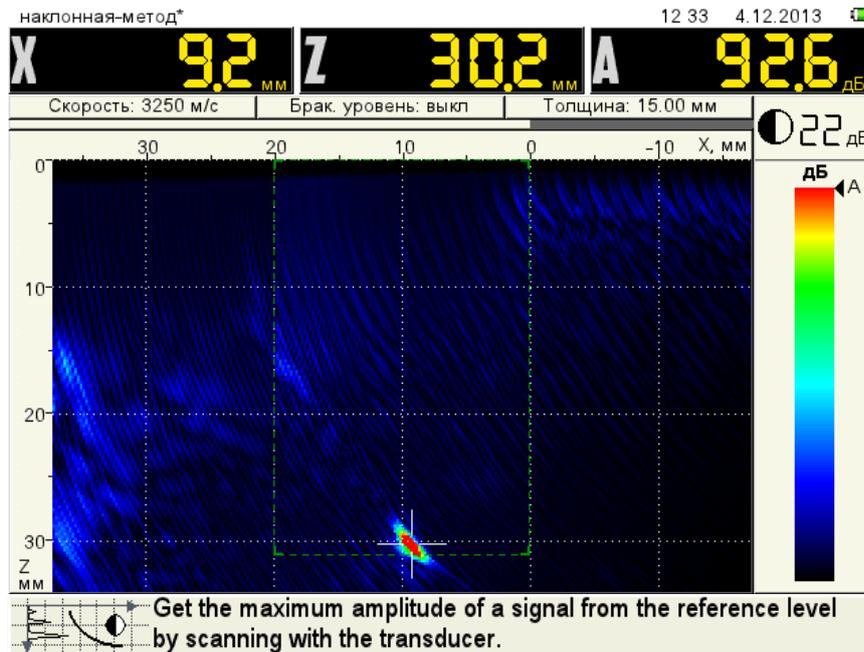
Figure 65 Determination of the reference level
