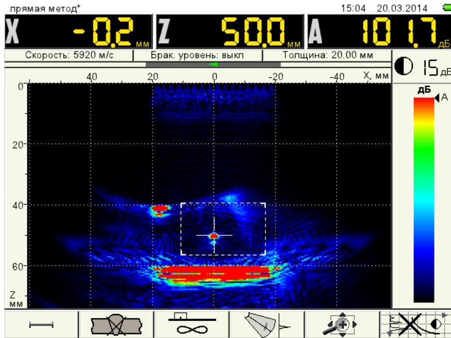
Figure 19 RR2. Depth Z2=50.0 mm, Amplitude A2=101.7 dB
