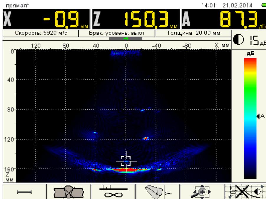
Figure 15 RR5 Depth Z5=150.3 mm, Amplitude A5=87.3 dB
