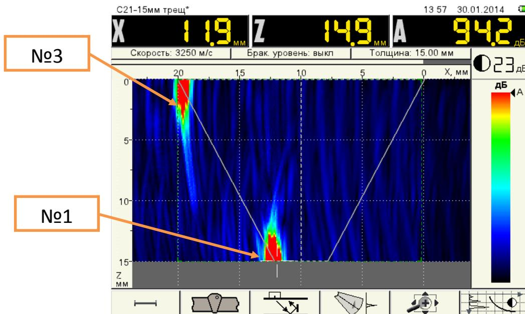
Figure 98 Vertical cracks mode. Images of the false reflectors
