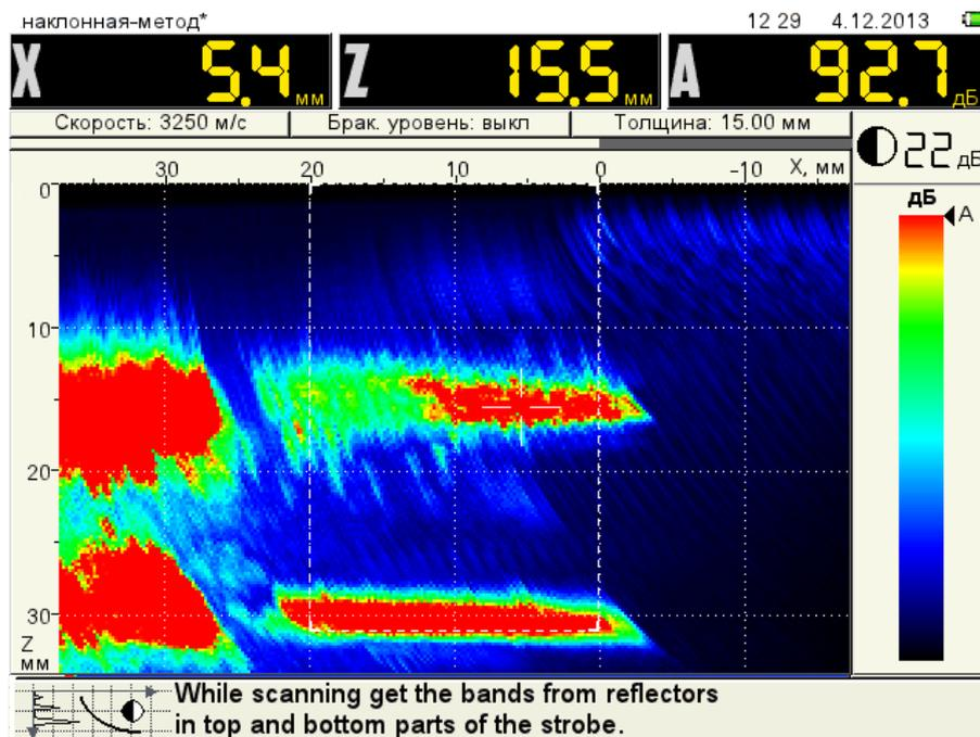
Figure 62 Adjustment of TCG by the distant reflector
