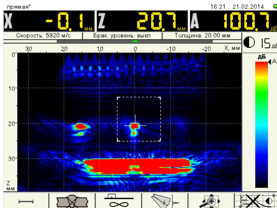
Figure 18 RR1. Depth  $Z_1=20.7$  mm, Amplitude  $A_1=100.7$  dB
