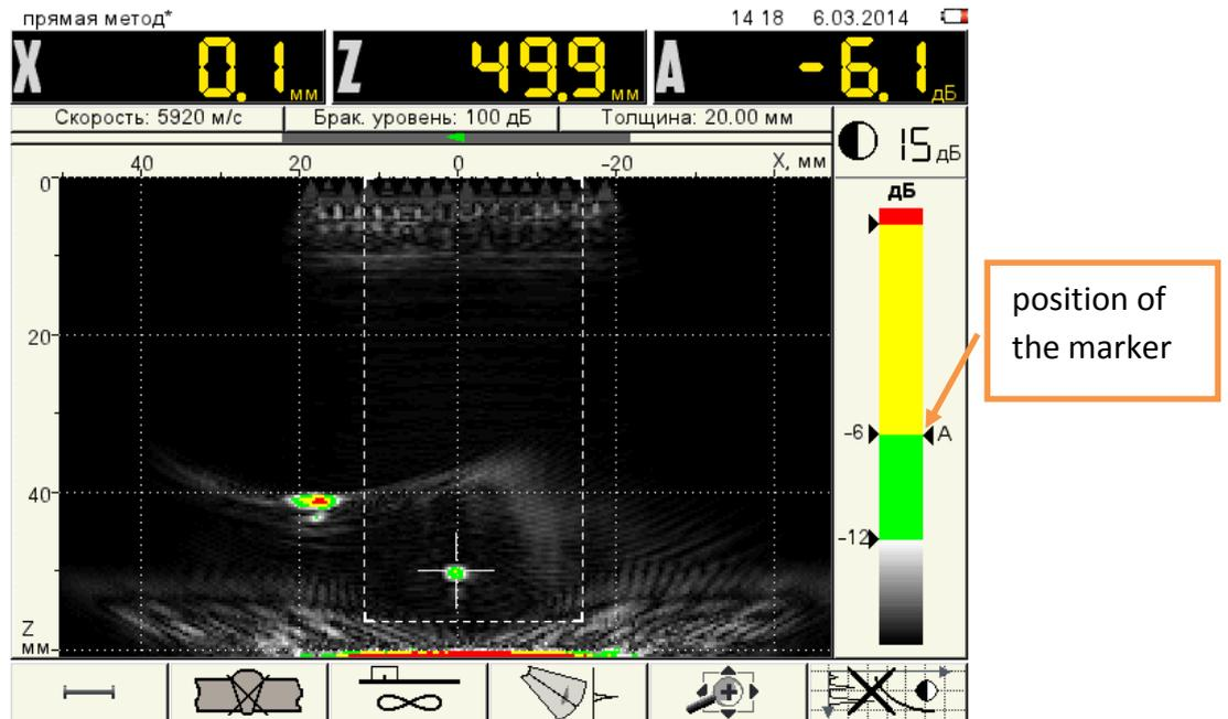
Figure 34 Image RR2 on the recording level -6 dB
