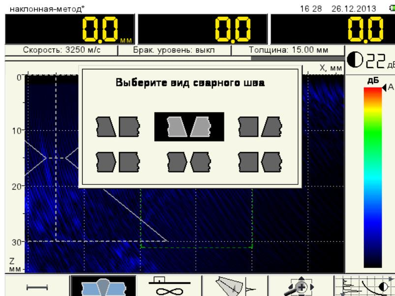
Figure 70 Selecting the welded seam
