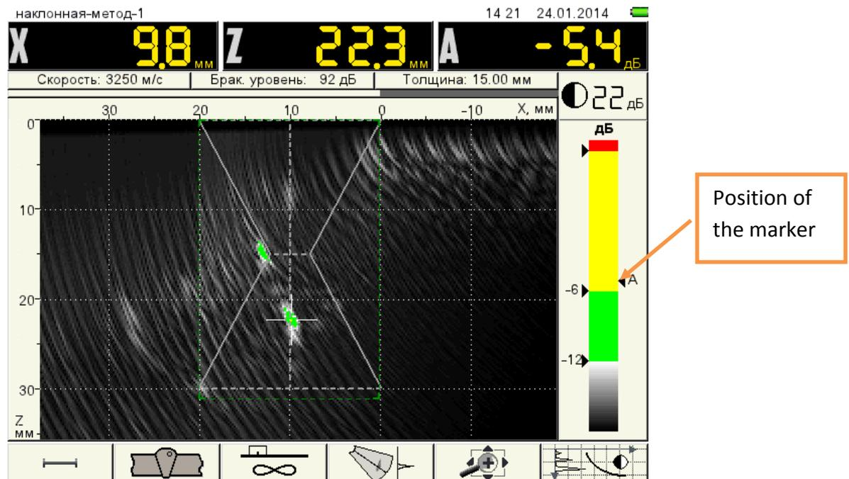
Figure 90 Determination of  $\Delta L$
