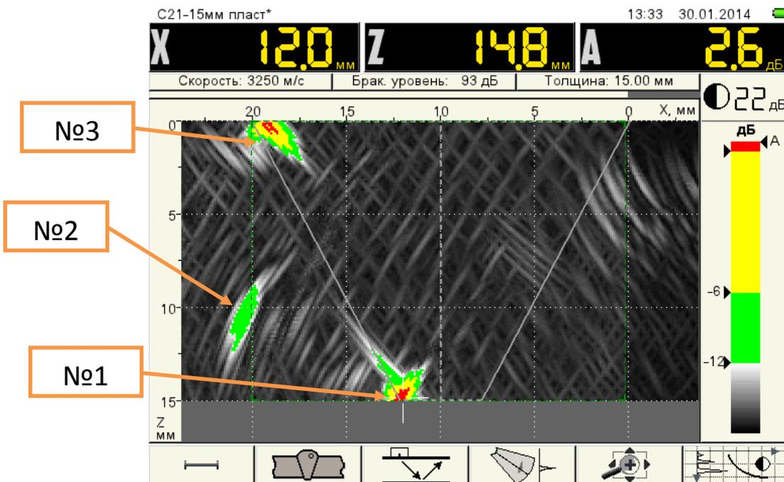
Figure 94 Plate mode. Images of the false reflectors
