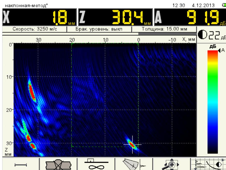
Figure 64 Checking TCG by the distant reflector
