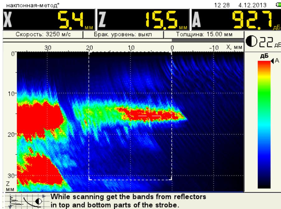
Figure 61 Adjustment of TCG to the near reflector
