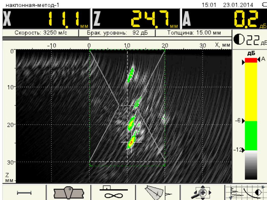
Figure 93 Images of the defects and false reflector
