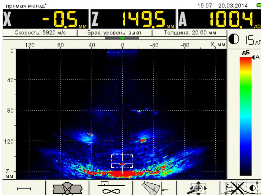
Figure 22 RR5. Depth Z5=149.5 mm, Amplitude A5=100.4 dB.
