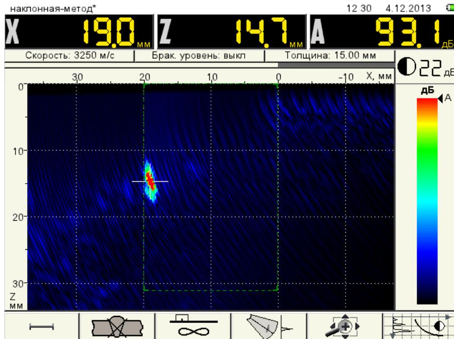
Figure 63 Checking TCG by the near reflector
