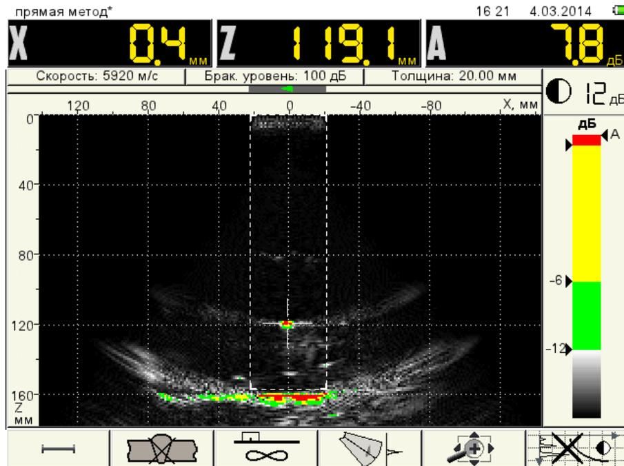
Figure 37 Image of defect at depth Z=119.1 mm
