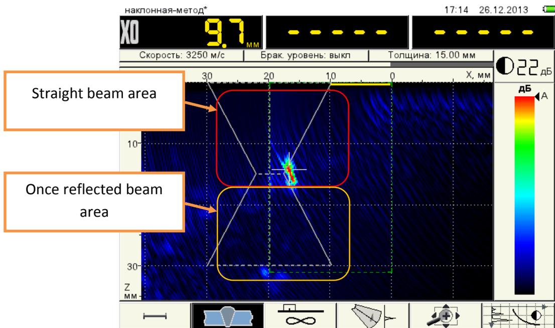
Figure 71 Setting the distance from the antenna array to the welded seam
