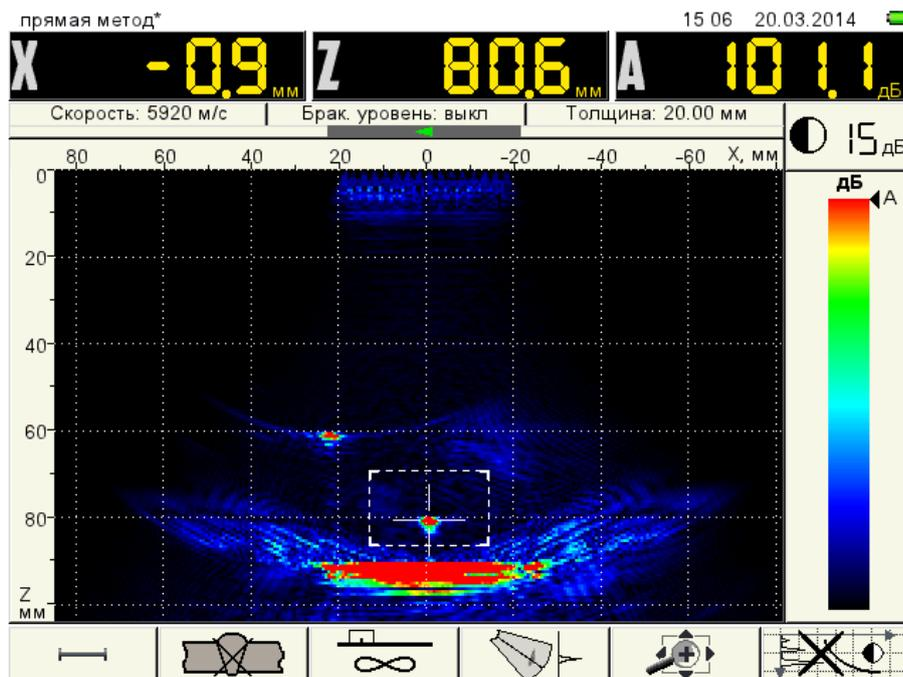
Figure 20 RR3. Depth Z3=80.6 mm, Amplitude A3=101.1 dB
