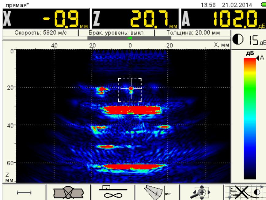
Figure 14 RR 1 Depth Z1=20.7mm, Amplitude A1=102 dB
