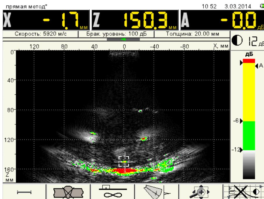
Figure 25 View of the operation mode with switched on reference level
