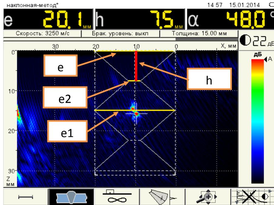
Figure 75 View of the welded seam image boundaries with double side edges and description of the measured parameters.
