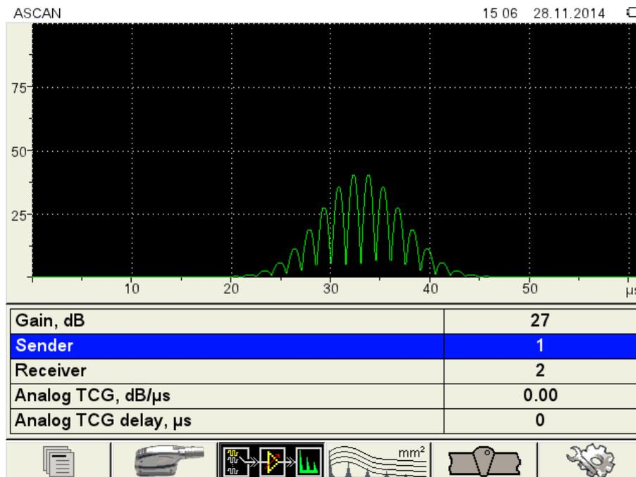
Figure 51 Adjustment of amplification of the 2.5 MHz frequency
