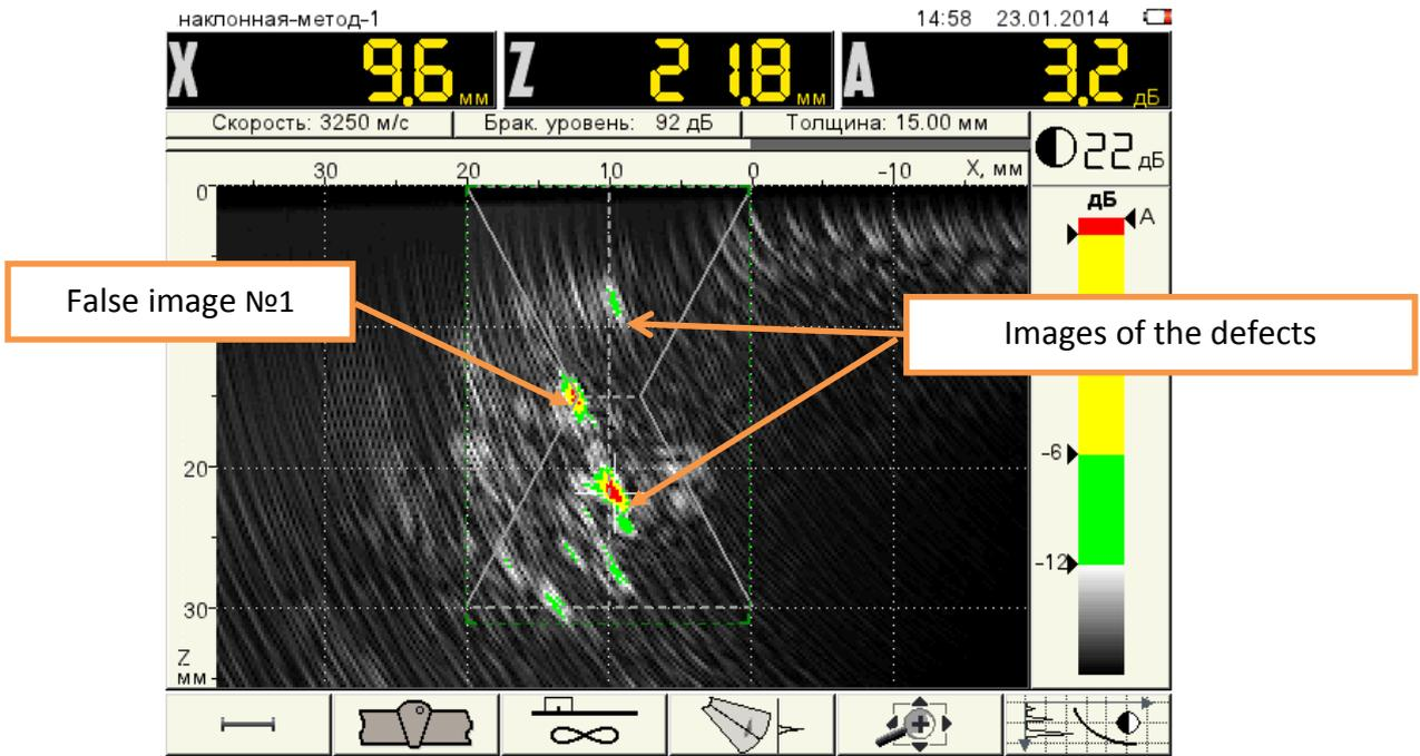
Figure 89 Images of the defect and false images
