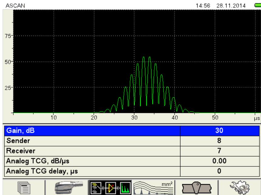
Figure 44 Configurations mode. Third tab
