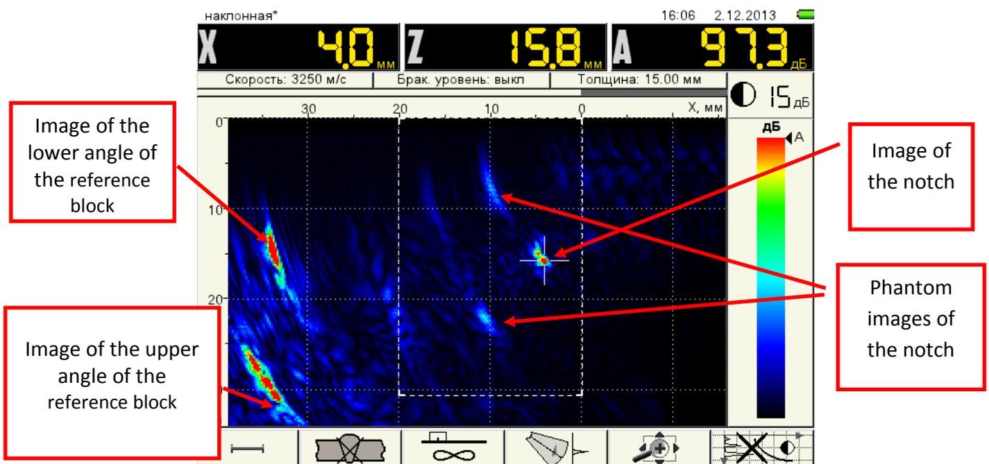
Figure 45 Operation mode. The antenna array is pointed to the near reflector
